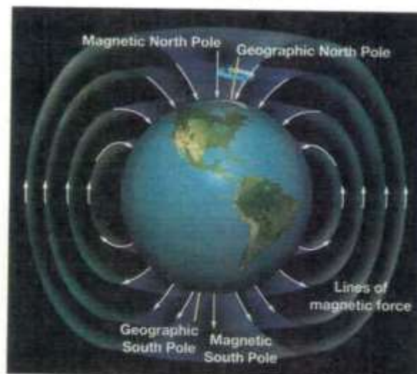
FIGURE 2.6 Earth's magnetic field is defined by magnetic lines of force shown by the arrows.
